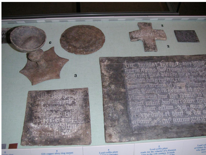
Fig 22. Lead coupon in showcase to check for pollution
