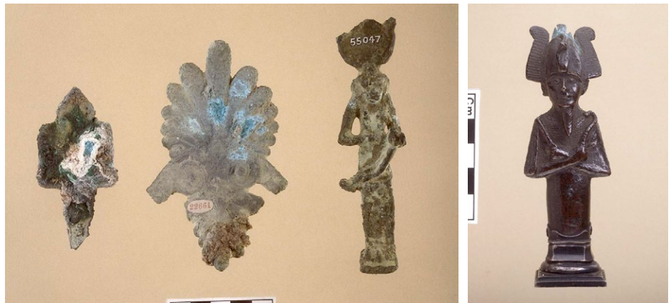
Fig 16 Copper alloy corrosion products containing sodium and carbonate as well as copper and acetate
