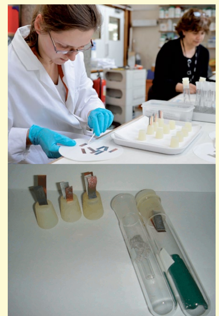
Fig 27. Oddy test being carried out © Museum of London
