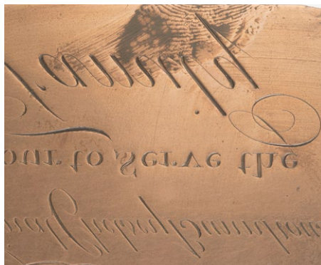
Fig 17. Detail of a copper alloy printing plate with corrosion from a fingerprint. © Museum of London
