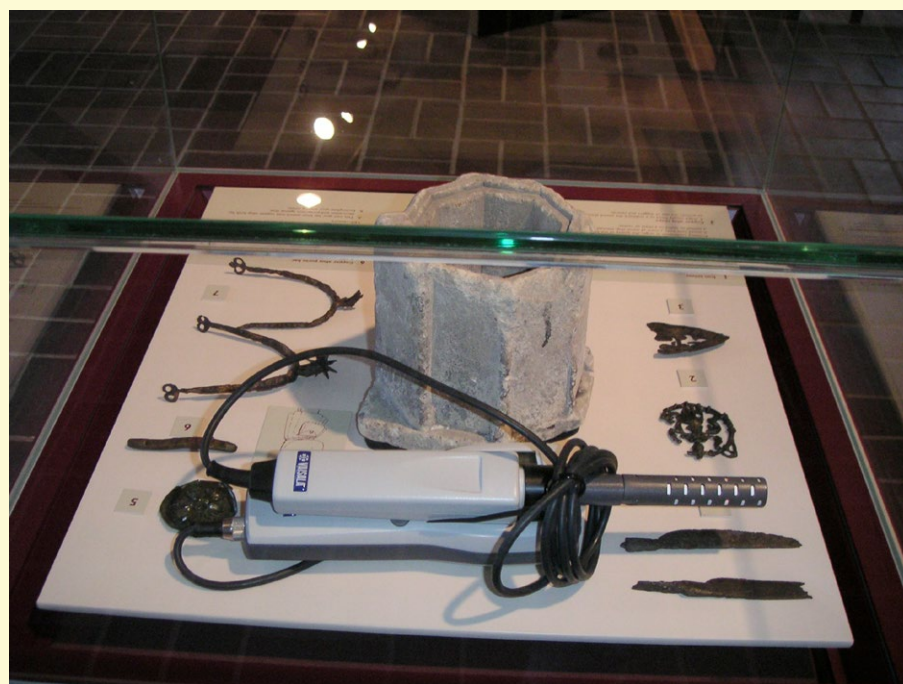
Fig 23. Measuring air exchange rate in a showcase
