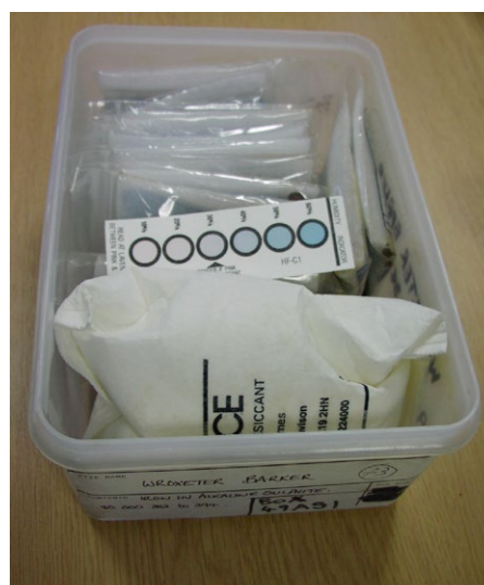
Fig 24. Stewart box for storing archaeological iron and copper alloy, with silica gel and RH indicator card
