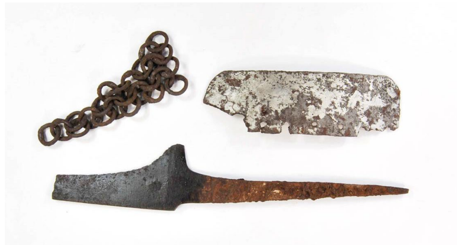
Fig 11. Iron from waterlogged sites in London showing excellent condition and typical corrosion layers; the blade is half-cleaned. © Museum of London
