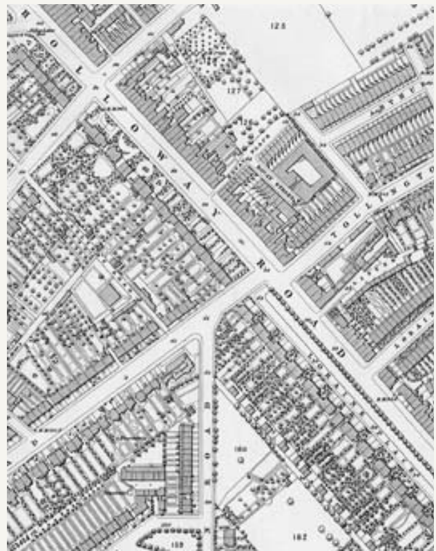
34 Ordnance Survey maps have been produced at a large scale since the 1860s and 1870s. This excerpt from a map of 1869 shows streets around Holloway Road, Islington, London; it is drawn at a scale of 1:2500.
